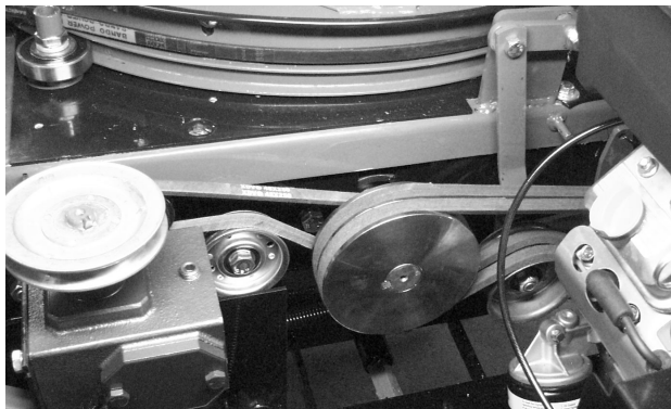
Figure 7 Rotor and Gear Box Drive Belt Installation
